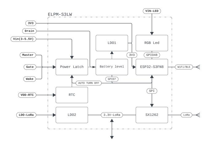
3V3: Main power path for the ESP32-S3FN8.
