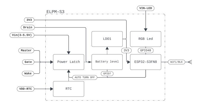
3V3: Main power path for the ESP32-S3FN8.
